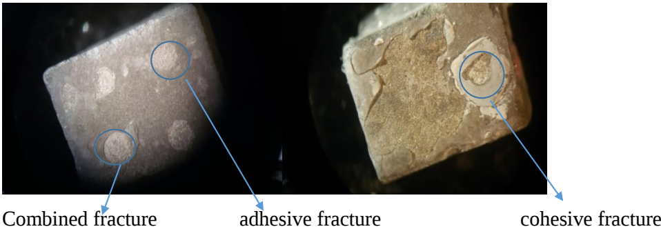
Figure 2. Different fracture patterns under a stereomicroscope
