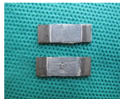
Figure 3. Broken specimens with/without soldering
