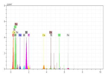
Fig. 2 A sample EDX spectrum of a bracket base composed of P, Ca, Si and Fe.
