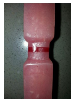
Figure 1. Acrylic specimens with 3mm wax in its narrowest part
