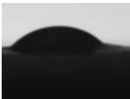
Fig. 1-Sessile drop of bonding agent on the dentin surface
