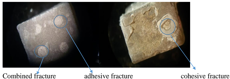
Figure 2. Different fracture patterns under a stereomicroscope
