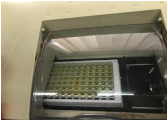
Figure 3. ELISA Plate Reader, in order to read the absorption of the wells
