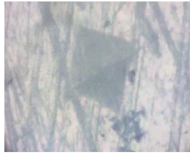
Figure 2: Hardness test sample and 200gf force
