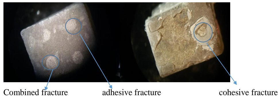
Figure 2. Different fracture patterns under a stereomicroscope
