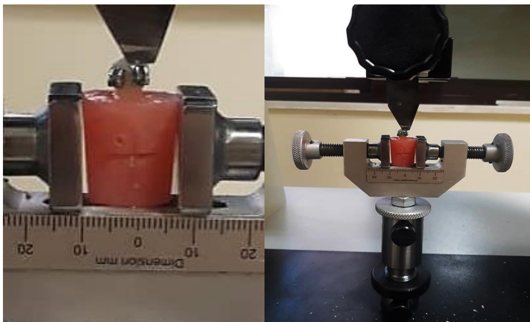
Figure 1. The position of the tooth sample in the machine to measure the shear bond strength of the bracket with composite resin to the tooth enamel
