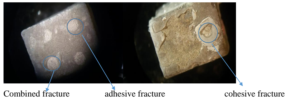
Figure 2. Different fracture patterns under a stereomicroscope
