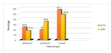
Figure 2. Comparison of the frequency of different failure types for the two groups
