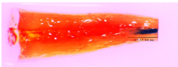
Fig5. A specimen of a measure of microleakage amount from the apical end in the horizontal dimension (2533 \mu\text{m} )
