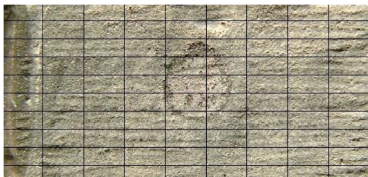
Figure 5. Broken specimen with soldering at x10.5 magnification
