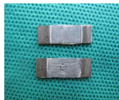
Figure 3. Broken specimens with/without soldering
