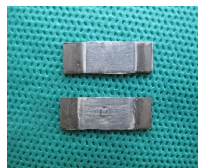
Figure 3. Broken specimens with/without soldering
