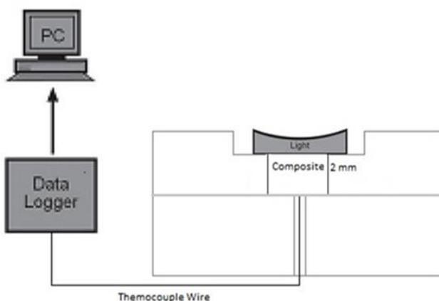
**Figure1. Schematic representation of the temperature rise measurement during polymerization of the composite resin material**
